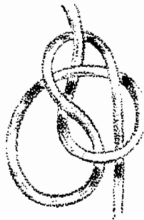
f Bowline. For making a non-slip loop in the end of a rope.
