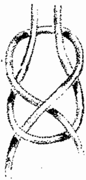
d Sheet Bend. For joining two ropes of unequal diameters.
